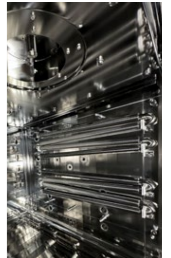
Internal cooling coils
