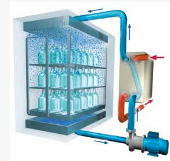
Hot water cascading process
